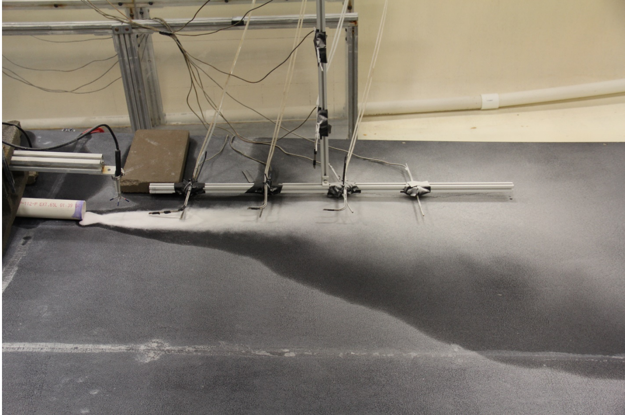
Fig. 38. Photograph of deposit for experiment 17. The current deposit is on the left close the pipe. The length/width ratio is large. The particles deposited on the right are the fall from the lofting plume. This is the case for all the lofting experiments.
