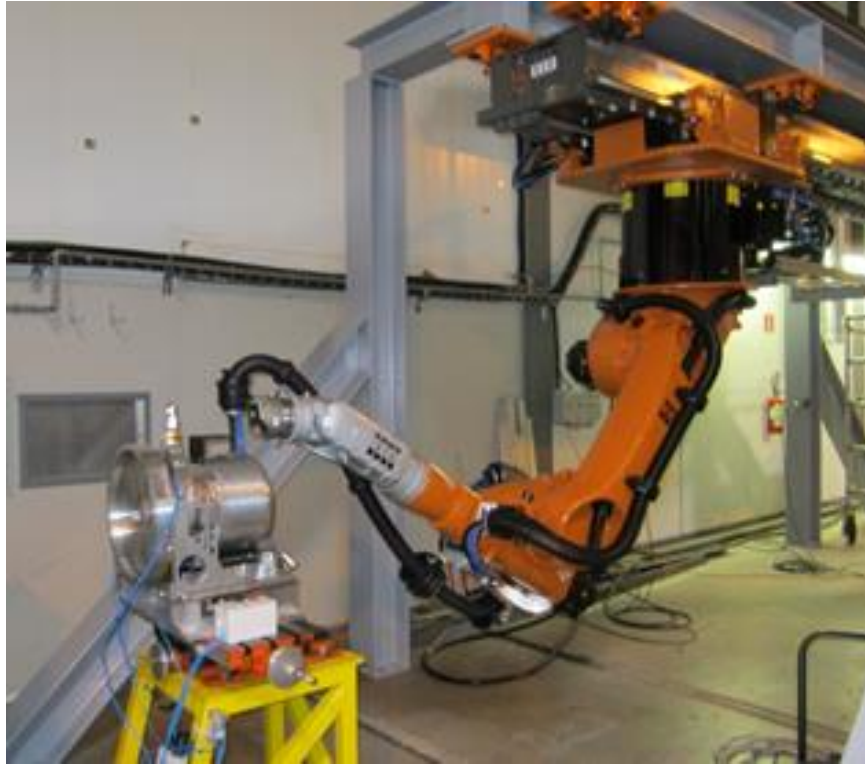
Figure 2-10. Target area with suspended robot at CERN. [Kershaw et al., 2013]
