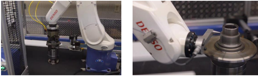
Figure 2-5. Operation of Univ-Versal dual-arm robotic eddy-current system. [UniWest, 2011]
