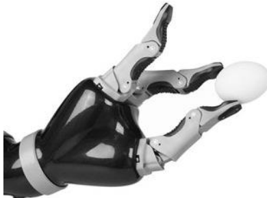
Figure 2-16. Example grasp of a Kinova JACO gripper. [Kinova, 2012]
