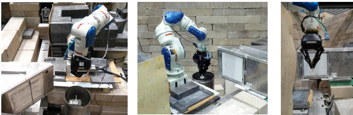
Figure 6-19. Robot demonstrating pick-and-place capability for a fuel rod placed inside of a canister.
