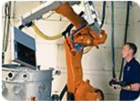
Figure 2-1. Robotic radiography inspection of a turbine case for a jet aircraft engine. The radiographic source is on one robotic arm and a digital detector on another. [Bosserman, 2007]
