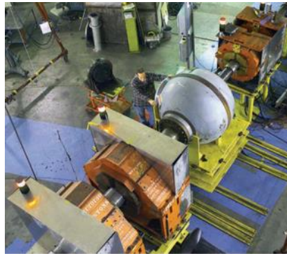
Figure 6-5. The pRad facility at LANSCE provides 50 ns wide H^- beam pulses with approximately 10^9 protons per pulse that are spaced in time intervals predetermined by experimental requirements. Transmitted and scattered protons are imaged by an electromagnetic lens system and recorded by a scintillator-mirror-camera system. A magnet magnifier lens provides a factor of 7 magnification for small systems with spatial resolution to roughly 15 \mu\text{m} . [Lacerda and Schoengberg, 2012]
