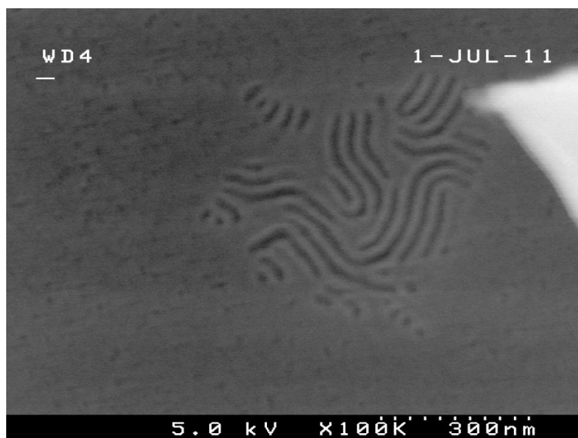
Figure 6.9: Initial hints that top coats may be effective at controlling block copolymer orientation. PS- b -PTMSS- b -PS film thickness was 44 nm ( 1.46 \cdot L_0 ) with a substrate surface treatment XST-OMe, annealed at 170°C for 19 hr 45 min.
