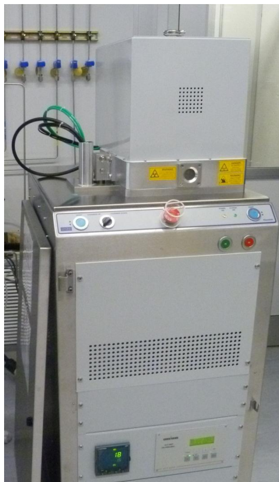
Figure 5.3: Oxford Plasmalab 80+ inductively coupled reactive ion etcher at UT-Austin used for the etch studies reported herein.
