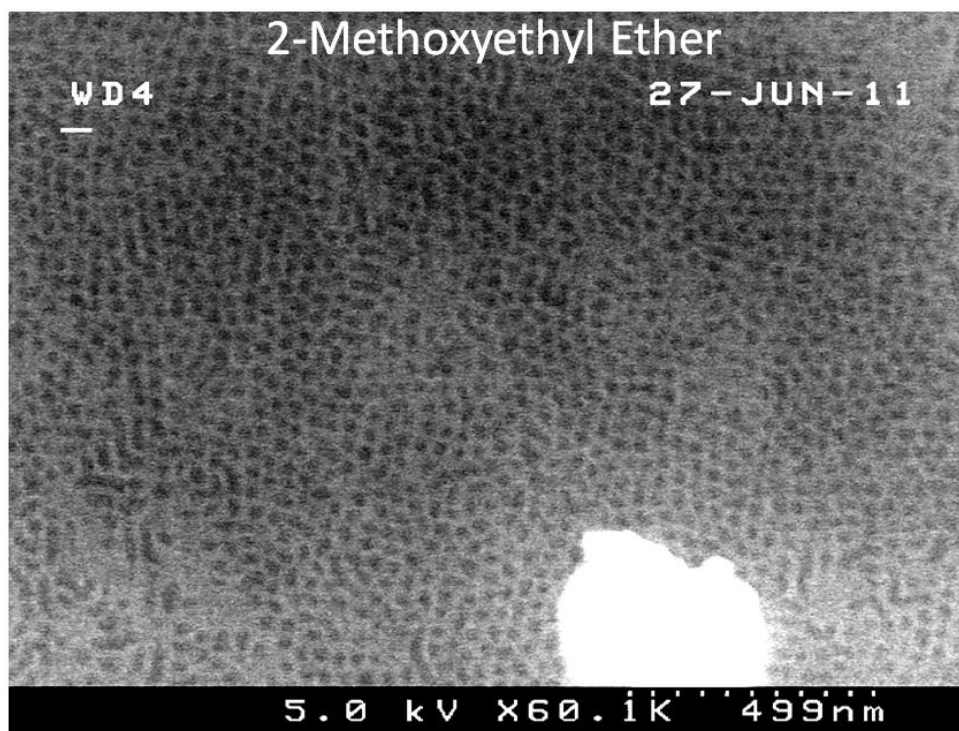
Figure 4.29: Larger field view of PS- b -PTMSS- b -PS solvent annealed for 1 h with 2-methoxyethyl ether.
