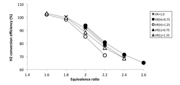
Figure 37. Hydrogen conversion efficiencies are shown for each of the scaled reactors, including those scaled by height (VR(h)=0.75 and VR(h)=1.25) and those scaled by length (VR(L)=0.75 and VR(L)=1.25), as a function of equivalence ratio at u = 125 cm/s.
