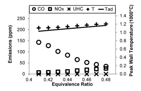
Figure 20. CO, NOx and UHC concentrations and peak wall temperature measurements (T), as well as adiabatic equilibrium temperature ( $T_{ad}$ ), for varying  $\phi$  with u = 125 cm/s
