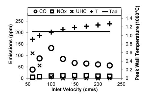
Figure 21. CO, NOx and UHC concentrations and peak wall temperature measurements (T), as well as adiabatic equilibrium temperature (T<sub>ad</sub>), for varying uand  $\phi = 0.44$
