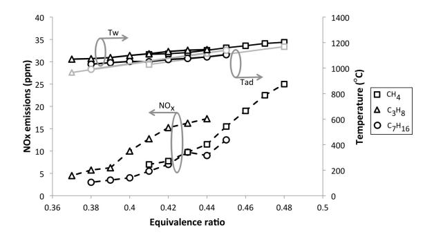
Figure 28. NO<sub>x</sub> exhaust concentration and peak wall temperature (Tw) measured for lean counter-flow combustor operation on heptane, propane and methane [39] with varying  $\phi$  and inlet velocity held constant at u = 125 cm/s are shown, as well as adiabatic equilibrium temperatures (Tad) calculated for the range of tested equivalence ratios of each fuel
