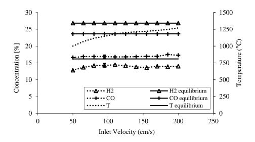
Figure 11. Exhaust gas and equilibrium concentrations of H<sub>2</sub> and CO, and peak wall and adiabatic equilibrium temperatures for  $\phi = 3.0$  and varying *u*
