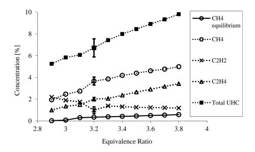
Figure 10. Exhaust gas concentrations of CH<sub>4</sub>, C<sub>2</sub>H<sub>2</sub>, C<sub>2</sub>H<sub>4</sub> and total UHC, and equilibrium concentrations of CH<sub>4</sub> (equilibrium concentrations of C<sub>2</sub>H<sub>2</sub> and C<sub>2</sub>H<sub>4</sub> are negligible and not shown) for u = 125 cm/s and varying  $\phi$
