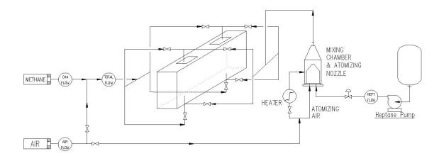
Figure 7. Vaporization and mixing chamber, and manifold piping to reactor inlets
