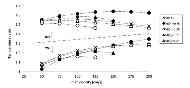
Figure 36. Separated by a dashed line, gas (above) and wall (below) temperature ratios are shown for each of the scaled reactors, including those scaled by height (VR(h)=0.75 and VR(h)=1.25), those scaled by length (VR(L)=0.75 and VR(L)=1.25), and original reactor geometry (VR=1.0), as a function of inlet velocity at  $\phi = 2.2$ .
