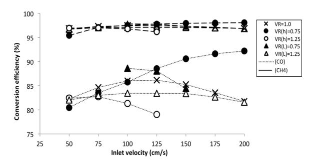
Figure 40. CO and CH<sub>4</sub> conversion efficiencies are shown for each of the scaled reactors, including original reactor geometry (VR=1.0), those scaled by height (VR(h)=0.75 and VR(h)=1.25) and those scaled by length (VR(L)=0.75 and VR(L)=1.25), as a function of inlet velocity at  $\phi = 2.2$ .
