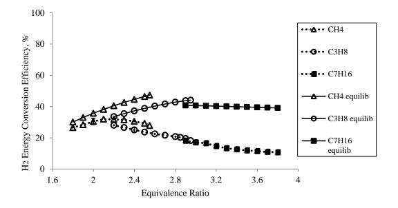
Figure 14. Experimental and equilibrium  $H_2$  energy conversion efficiencies of methane [36], propane [37] and heptane reforming with constant u = 125 cm/s and varying equivalence ratio
