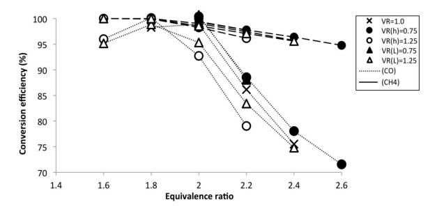
Figure 39. CO and CH<sub>4</sub> conversion efficiencies are shown for each of the scaled reactors, including original reactor geometry (VR=1.0), those scaled by height (VR(h)=0.75 and VR(h)=1.25) and those scaled by length (VR(L)=0.75 and VR(L)=1.25), as a function of equivalence ratio at u=125 cm/s.
