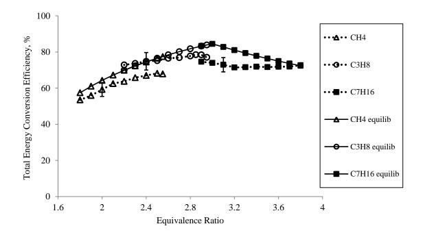
Figure 15. Experimental and equilibrium total energy conversion efficiencies of methane [36], propane [37] and heptane reforming with constant u = 125 cm/s and varying equivalence ratio
