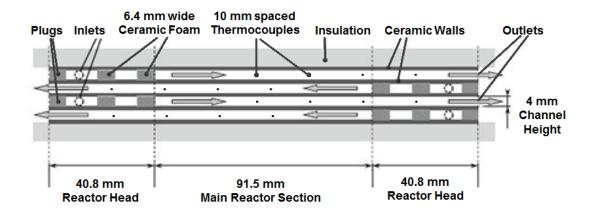
Figure 5. Counter-flow reactor schematic with components and dimensions
