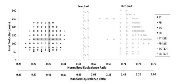
Figure 23. Stability map for counter-flow reactor operation on lean and rich [37] propane/air reactants, with stable (ST) and unstable points due to flashback (FB), blow-off (BO) and extinction (EX) shown as a function of inlet velocity and both standard and normalized equivalence ratios. Lean and rich flammability limits for propane/air reactants at inlet conditions are indicated.
