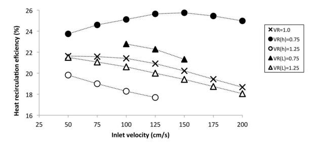
Figure 34. Heat recirculation efficiency is shown for each of the scaled reactors, including those scaled by height (VR(h)=0.75 and VR(h)=1.25) and those scaled by length (VR(L)=0.75 and VR(L)=1.25), as a function of inlet velocity at  $\phi = 2.2$ .
