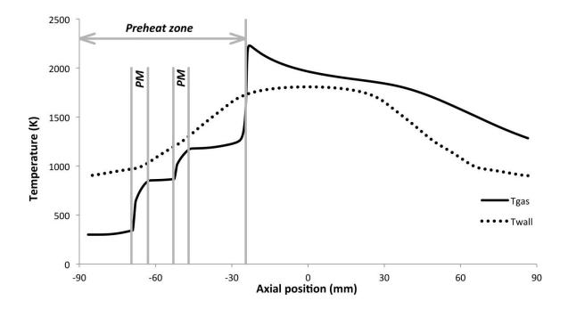
Figure 32. Gas (Tgas) and wall (Twall) temperature profiles along the axial length of a counter-flow reactor channel, obtained from the original reactor geometry (VR=1.0) with inlet conditions of  $\phi = 2.2$  and u = 125 cm/s. The preheat zone is identified, as well as the locations of the two sections of porous media flow straighteners (PM), the high thermal conductivity of which contributes to preheating the reactants.
