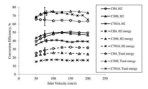
Figure 16. H<sub>2</sub>, H<sub>2</sub> energy and total energy conversion efficiencies of methane ( $\phi = 2.2$ ) [36], propane ( $\phi = 2.4$ ) [37] and heptane ( $\phi = 3.0$ ) with varying inlet velocity
