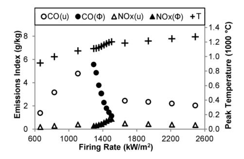
Figure 22. Emission indices of CO (EICO) and NOx (EINOx), and peak reactor wall temperature (T) over a range of tested firing rates for the variation of equivalence ratio ( $\phi$ ) and inlet velocity (u)
