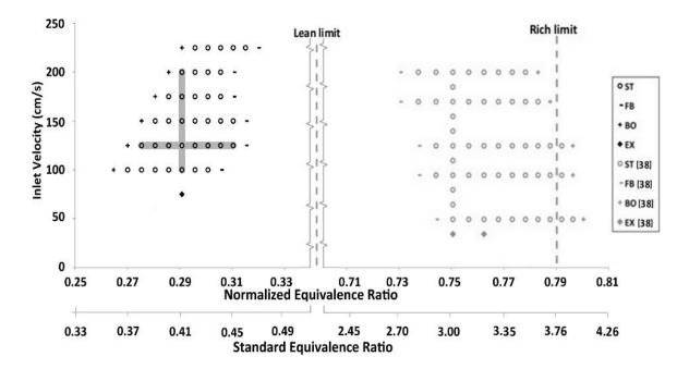
Figure 24. Stability map for counter-flow reactor operation on lean and rich [38] heptane/air reactants, with stable (ST) and unstable points due to flashback (FB), blow-off (BO) and extinction (EX) shown as a function of inlet velocity and both standard and normalized equivalence ratios. Lean and rich flammability limits for heptane/air reactants at inlet conditions are indicated.
