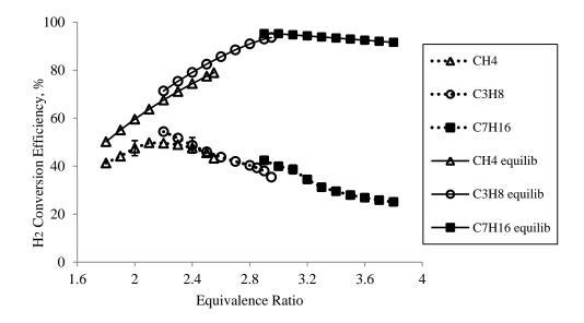
Figure 13. Experimental and equilibrium values of  $H_2$  conversion efficiencies of methane [36], propane [37] and heptane reforming with constant u = 125 cm/s and varying equivalence ratio
