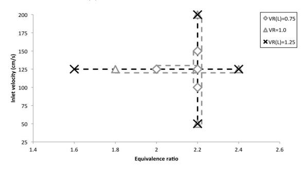
Figure 31. Operating range for counter-flow reactors scaled to smaller and larger volume ratios by varying channel length, VR(L)=0.75 and VR(L)=1.25, and original reactor geometry, VR=1.0, over the tested range of inlet velocities, u = 50-200 cm/s at  $\phi = 2.2$ , and the tested range of equivalence ratios,  $\phi = 1.4-2.6$  at u = 125 cm/s.
