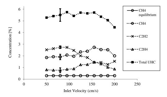
Figure 12. Exhaust gas concentrations of CH<sub>4</sub>, C<sub>2</sub>H<sub>2</sub>, C<sub>2</sub>H<sub>4</sub> and UHC, and equilibrium concentrations of CH<sub>4</sub> (equilibrium concentrations of C<sub>2</sub>H<sub>2</sub> and C<sub>2</sub>H<sub>4</sub> are negligible and not shown) for  $\phi = 3.0$  and varying *u*
