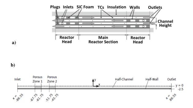
Figure 29. (a) A schematic of the four-channel reactor and (b) the computational domain of the original reactor geometry (VR=1.0)
