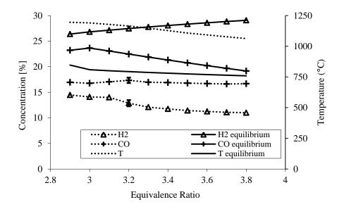
Figure 9. Exhaust gas and equilibrium concentrations of H<sub>2</sub> and CO, and peak wall and adiabatic equilibrium temperatures for u = 125 cm/s and varying  $\phi$
