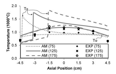
Figure 19. Analytical model (AM) gas ( $T_g$ ) and wall ( $T_w$ ) temperatures and experimental (EXP) temperatures measured along axial position in channel for varying *u* and  $\phi = 0.44$
