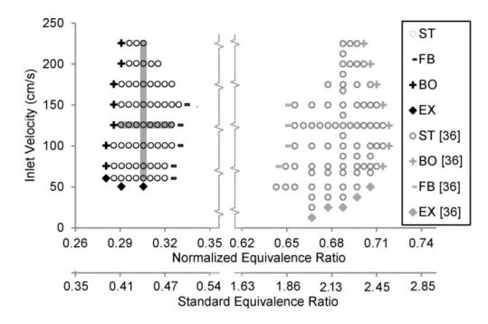
Figure 17. Stability map for counter-flow reactor operating on lean (this study) and rich ([36]) methane/air reactants, with both stable (ST) and unstable points due to flashback (FB), blow-off (BO) and extinction (EX) shown as a function of inlet velocity and both standard and normalized equivalence ratios
