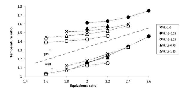
Figure 35. Separated by a dashed line, gas (above) and wall (below) temperature ratios are shown for each of the scaled reactors, including those scaled by height (VR(h)=0.75 and VR(h)=1.25), those scaled by length (VR(L)=0.75 and VR(L)=1.25), and original reactor geometry (VR=1.0), as a function of equivalence ratio at u = 125 cm/s.
