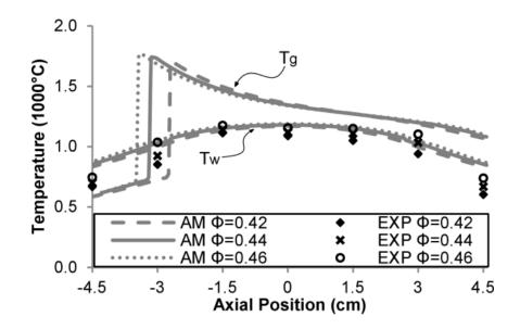
Figure 18. Analytical model (AM) gas ( $T_g$ ) and wall ( $T_w$ ) temperatures and experimental (EXP) temperatures measured along axial position in channel for varying  $\phi$  and u = 125 cm/s
