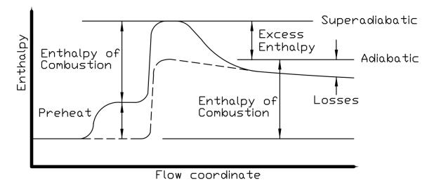
Figure 1. Combustion gas sensible enthalpy along flow coordinate with (solid line) and without (dashed line) heat recirculation
