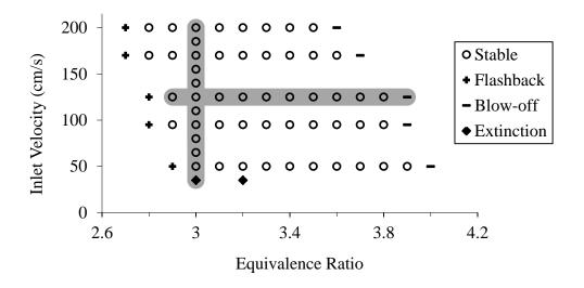
Figure 8. Stable and unstable operating conditions, with highlighted operating points where exhaust gas composition was analyzed
