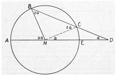
Required: to divide the arc AB of the circle with center M into three equal parts. Draw the diameter AE, and through B draw a secant cutting the circumference in C and the diameter AE in D, so that CD equals the radius r of the circle. Then
