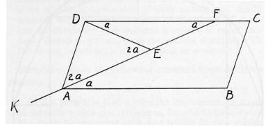
A simple instrument for trisecting an angle is made of four rods hinged together forming a collapsible parallelogram ABCD. A rod DE equal in length to AD is hinged at D and also to another rod KF at E. The rod KF has EF equal to AD, and the extremity F is allowed to move along DC by means of a ring.
