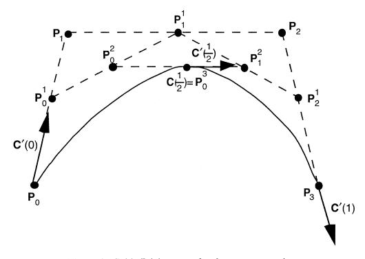
Figure 4. Cubic Bézier control polygon construction.
