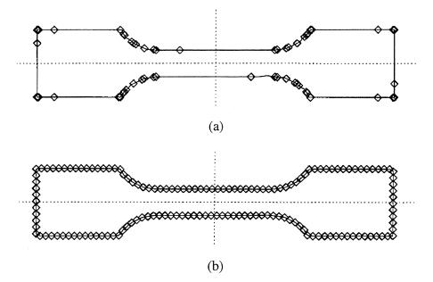
Figure 6. Cubic NURBS representation of the contour from Figure 3.
