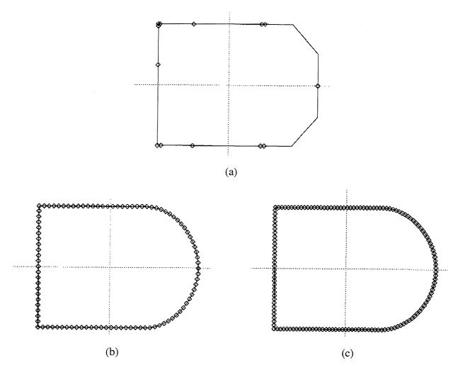
Figure 5. Given data and developed control polygon (a), and NURBS representation by Bézier algorithm with 100 points (b) and 150 points (c).
