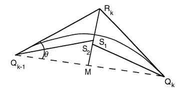
Figure 2. Determining the weight for a curve segment.
