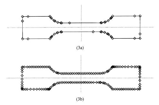
Figure 3. Original CAD data and developed control polygon (a), and NURBS representation by quadratic algorithm (b). (◊ indicates points given or calculated.)
