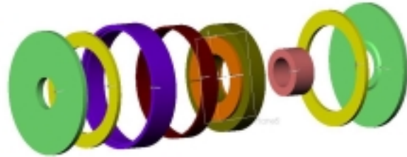
FIGURE 11. Exploded View of Combination Bearing Components
