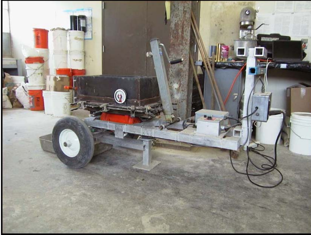
Figure 3.3 Vibrating Slope Apparatus Ready for Use
