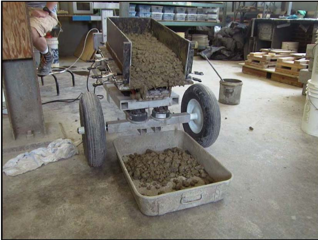
Figure 3.1 Concrete Sample Discharging From Chute under Vibration during Test
