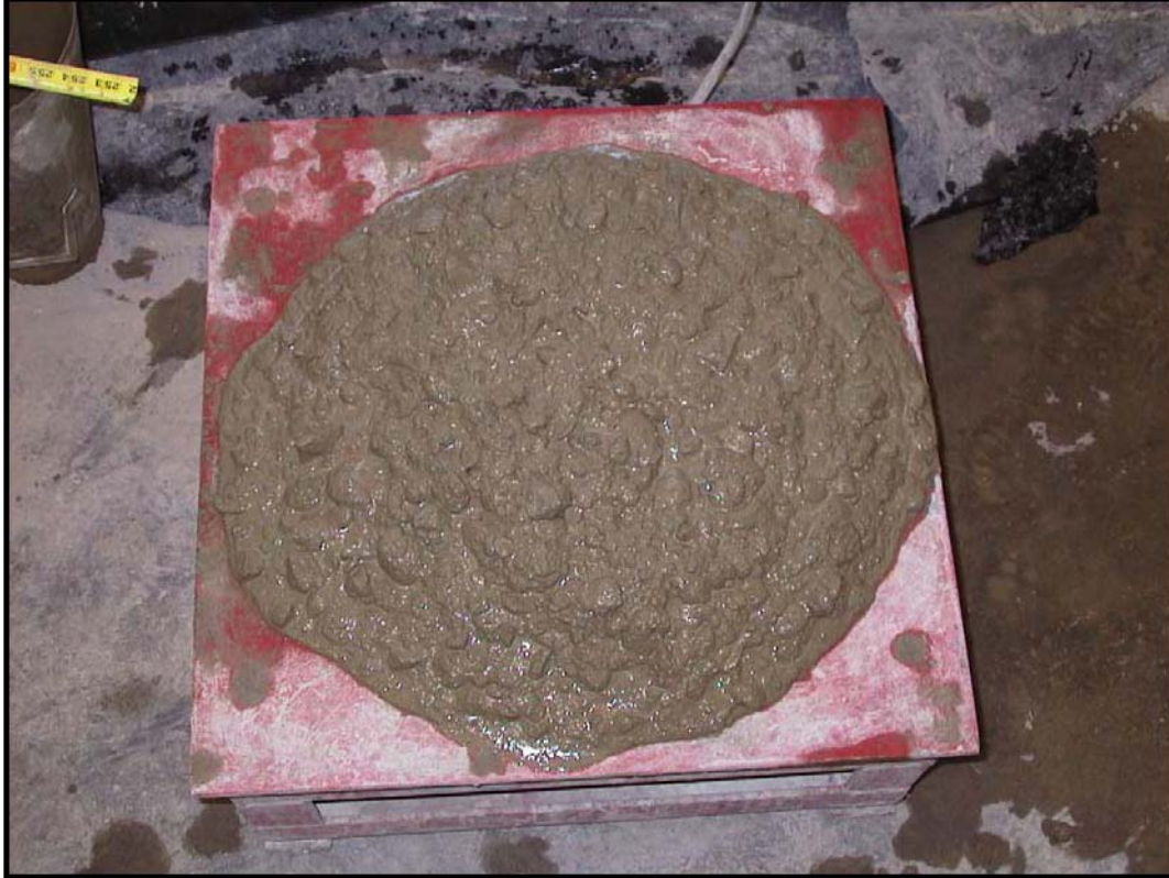
Figure 4.6 Slump Flow of Mixture 1 on July 18, 2003, an Initial 1.5-inch Slump, after 20 Seconds on Vibrating Table
