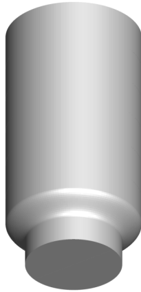
Figure 7.13: The shape of the fluid subproblem domain, \Omega_1 , defined by applying the transformation (7.5)–(7.7) to a trivariate B-spline parameter space.
