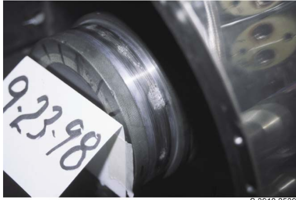
Figure 2. Brush arrangement on shaft of model scale compulsator
