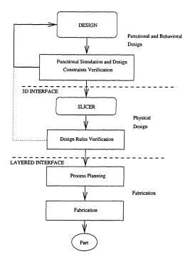
Figure 1: Design Hierarchy for Solid Freeform Fabrication
