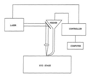
Figure 2: Laser-Aided Manufacturing of Multigraded Components
