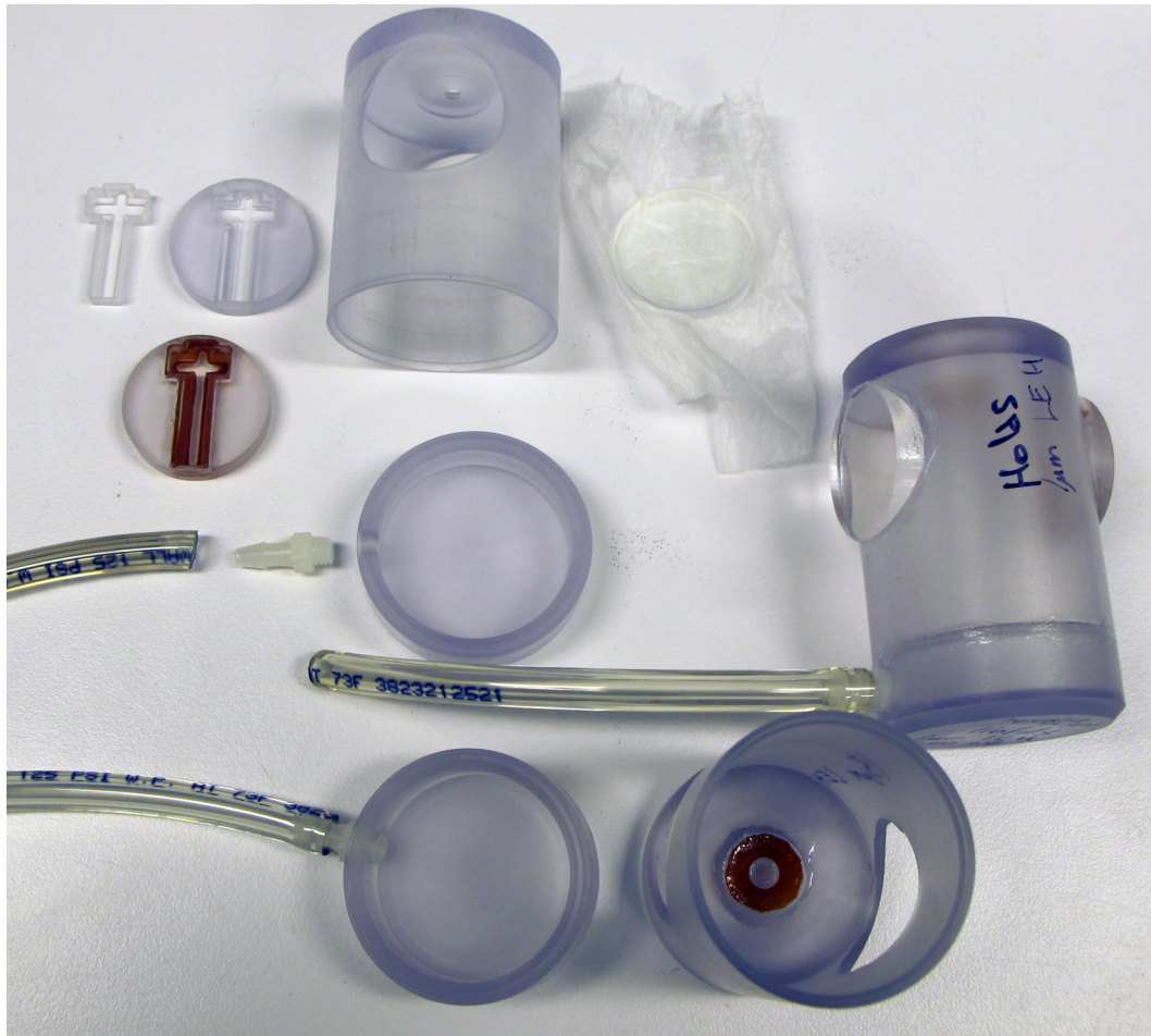
Figure 2.5: I assembled gas cells from raw parts from 2014 to 2016. 2 micron thick LEW and x-ray windows needed to be glued onto inserts and washers. We then attached these parts to the gas cell. Optical quality polycarbonate 1 inch windows came separately and needed to be glued on also. The hose barb connections for the fill lines are a stock part from McMaster-Carr company and needed to be glued on also. Pictured on the right is a completed gas cell target.
