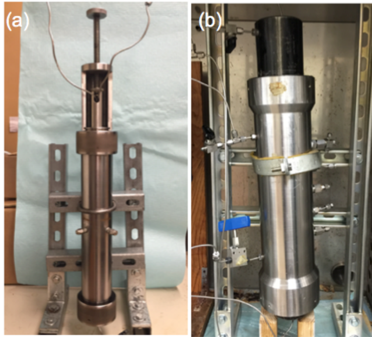
Figure 2.14: Specifications of the 12''-long steel coreholders manufactured by Phoenix Instruments (a) 1'' diameter Hassler coreholder (working pressure: 1250 psi), and (b) 2'' diameter Hassler coreholder (working pressure: 5000 psi).
