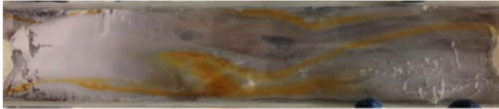
Figure 3.41: Hydrochloric acid (pH 2.29) pre-flushed cement core (6FP-27) after 24 hours polymer shut-in. White calcium precipitation with rust-colored precipitate (Patterson, 2014).
