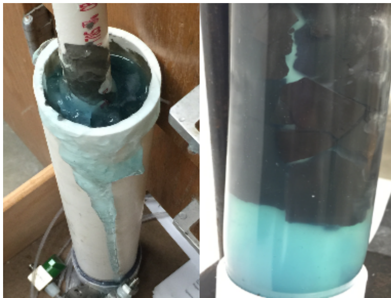
Figure 3.33: Experiment PVC-1 (left) and TYG-1 (right) successfully held 15 psi/ft constant pressure for one week. During pressure breakthrough test, PVC-1 had maximum breakthrough at 63 psi/ft and TYG-1 (right) had maximum breakthrough at 25.6 psi/ft.
