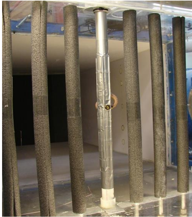
Figure 2.15: Wax sprayer in the wind tunnel replaces one of the turbulence rods
