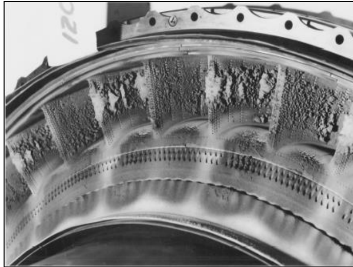
Figure 1.8: Volcanic ash deposition on gas turbine vane surface (Hamed, et al., 2006)
