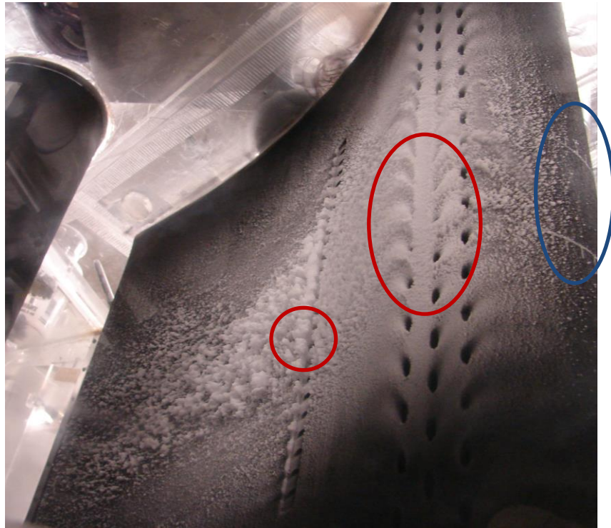
Figure 5.1: Vane model after deposition test viewing the leading edge and pressure side of the vane
