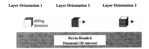
No significant anisotropy effect was observed in the abrasive wear values.
