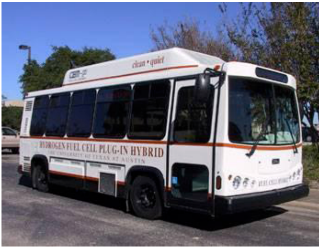
Fig. 1. Plug-in hybrid fuel cell bus manufactured by Ebus
