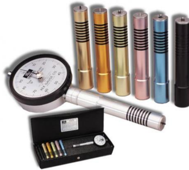
Figure 3.9: Durometer and scales for Brinell hardness test.
