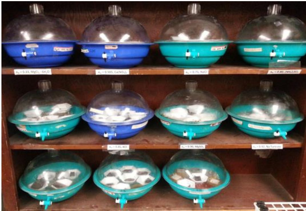
Figure 3.4: Desiccators for measuring water activity of shale.
