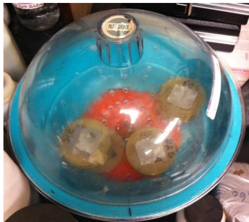
Figure 3.5: Shale samples on a plate in desiccators (Zhou et al. 2013).
