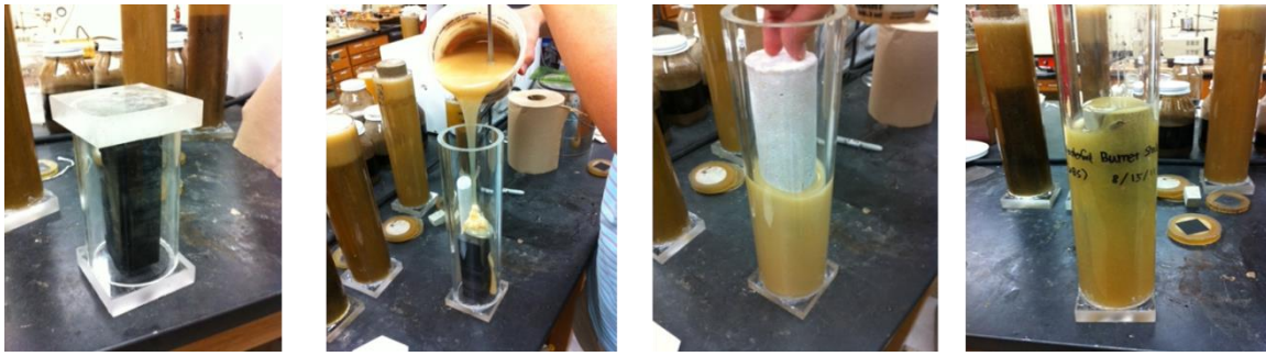
Figure 4.10: Epoxy resin encapsulating the shale core.
