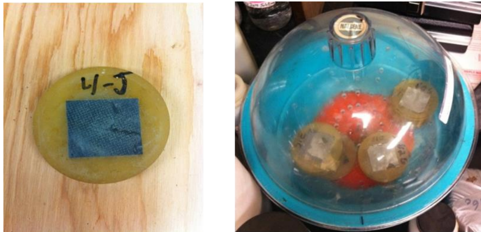
Figure 4.11: Sliced disk type sample (left) and a desiccator containing properly saturated salt (right).
