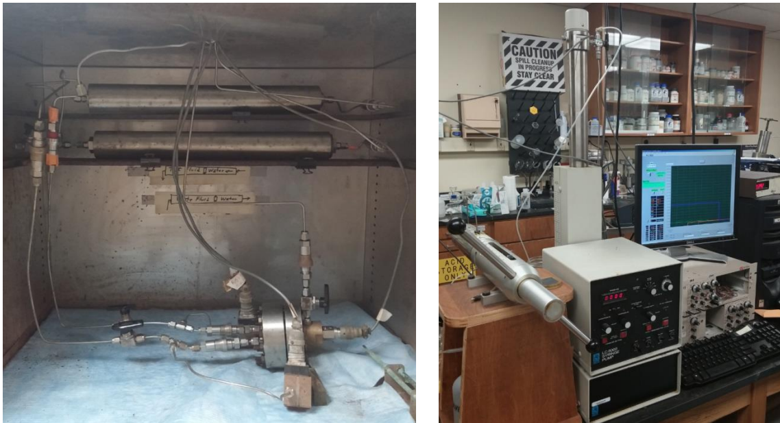
Figure 4.2: Pressure penetration test set-up.
