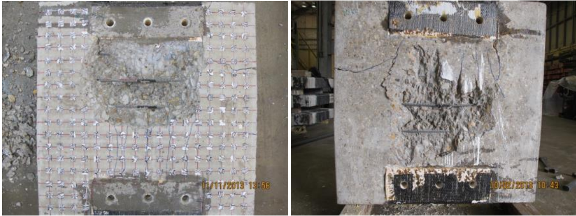
(a) Concrete crushing of front side
