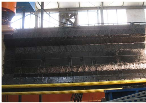
(c) Bi-directional fully wrapped beam
