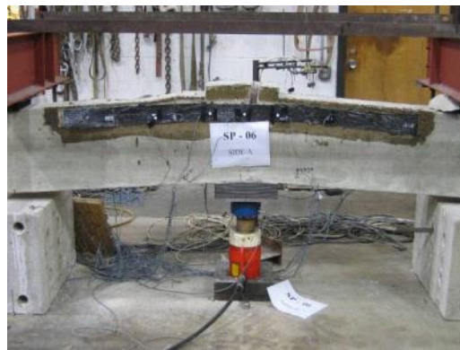
(b) Beam with CFRP anchors
