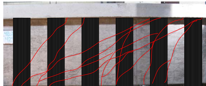
(b) Example of uni-directional CFRP layout
