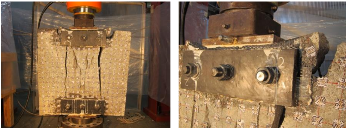
Figure 4.9 Failure mode of specimen C0-0-0-11
