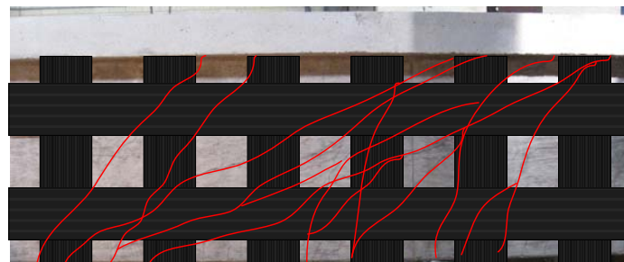
(c) Example of bi-directional CFRP layout
