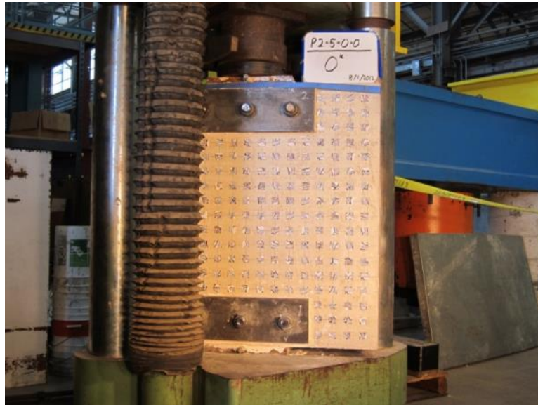
Figure 4.6 C0-0-0-5 panel in the universal testing machine, UTM
