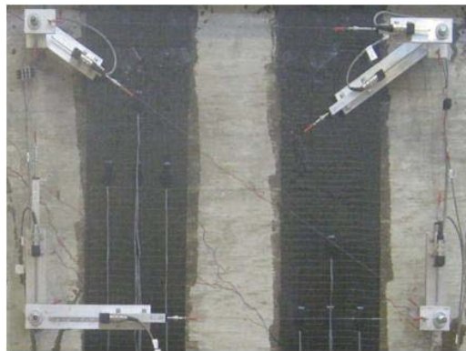
Figure 2.5 LVDTs configuration for shear strain calculation (Kim, 2011)
