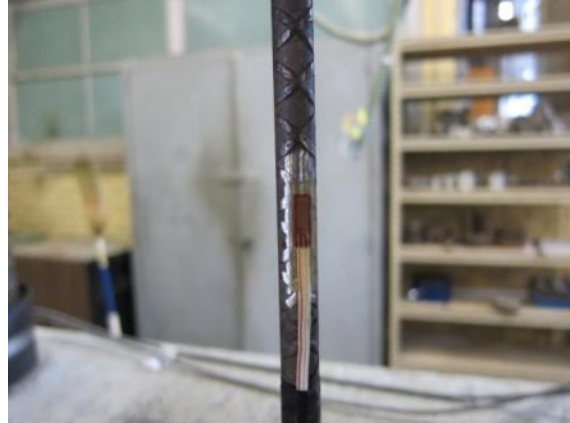
(b) Strain gage on the bar
