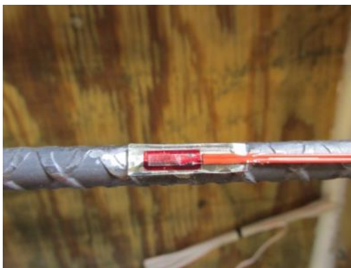
(c) Strain gage on the rebar
