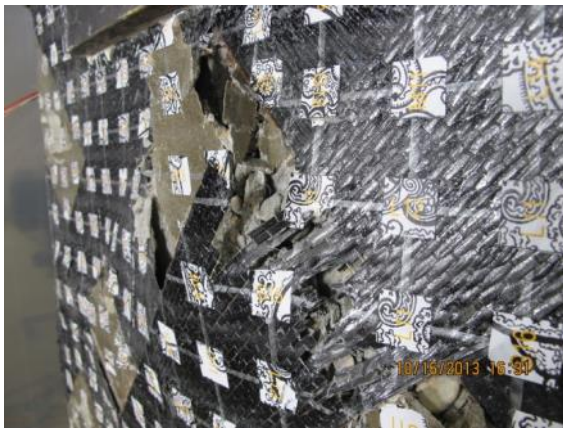
(c) Failure mode of B5-45-2-5
