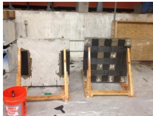
(f) Panels after the CFRP application
