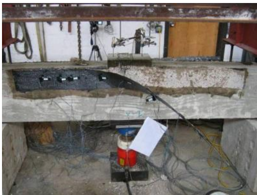
(a) Beam without CFRP anchors
