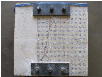
(c) Crack pattern
