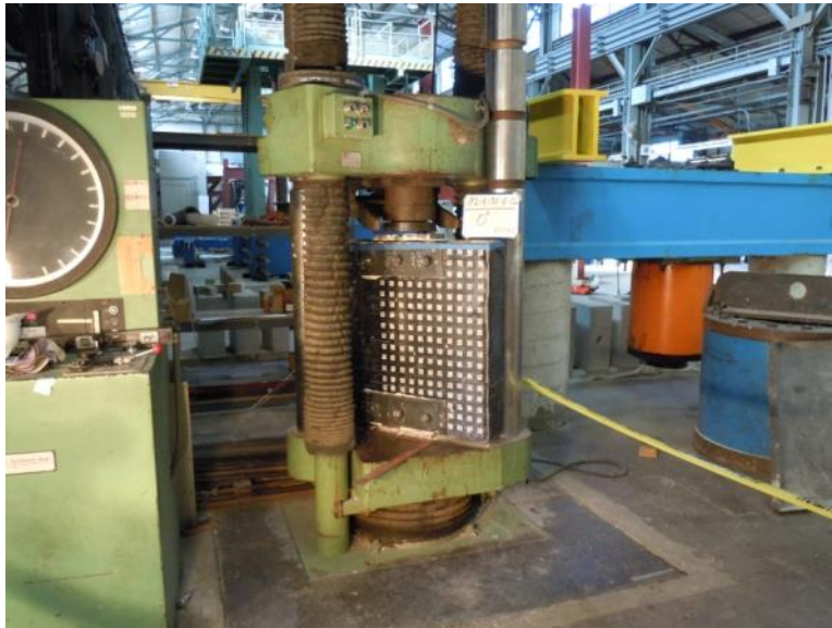
Figure 3.11 600 kips Universal Testing Machine (UTM)
