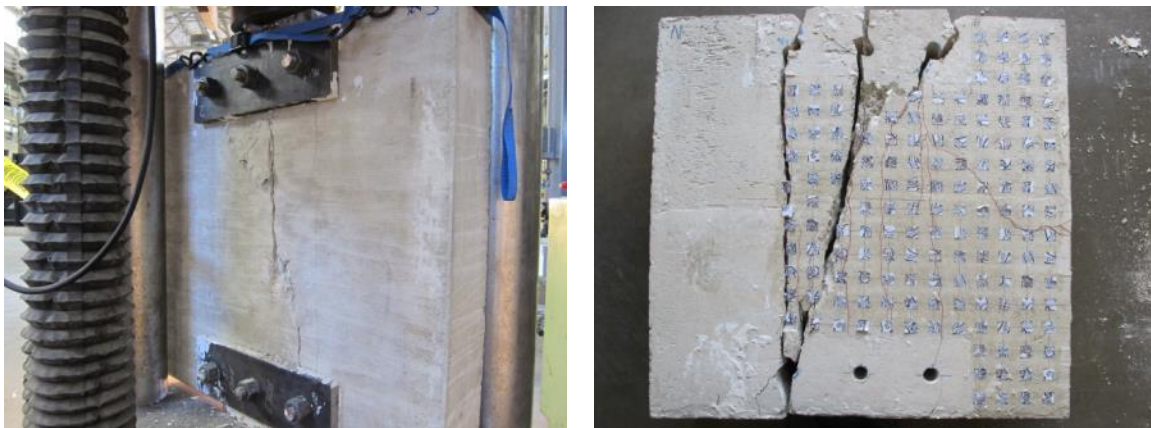
Figure 4.7 Failure mode of specimen C0-0-0-5
