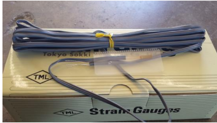
Figure 3.16 Steel strain gage
