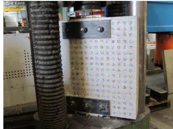
(b) Steel plates on the panel
