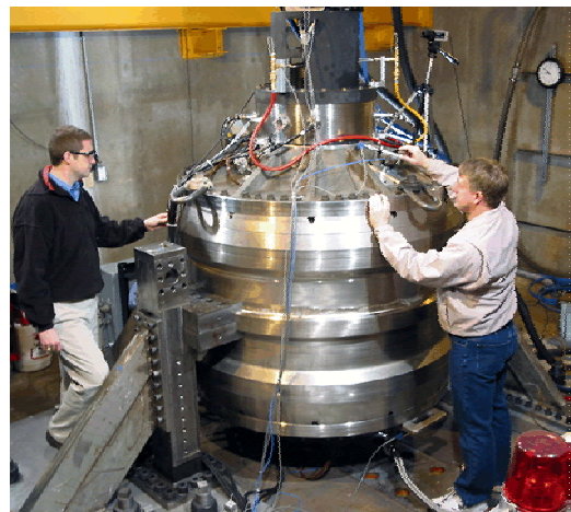
Figure 6. ALPS Flywheel undergoing spin testing.
