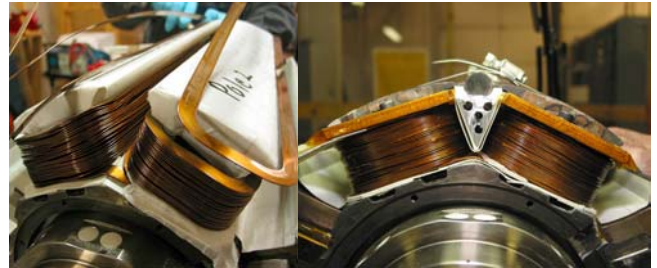
Figure 5. Field winding and cutaway of oil cooling wedge.
