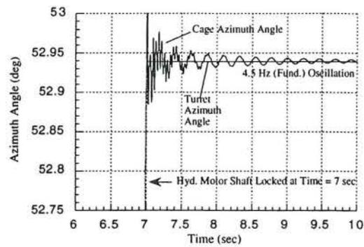
Figure 7: Azimuth Braking
