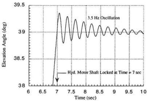
Figure 6: Elevation Braking
