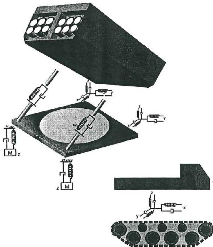
Figure 2: Mechanical Assembly Model
