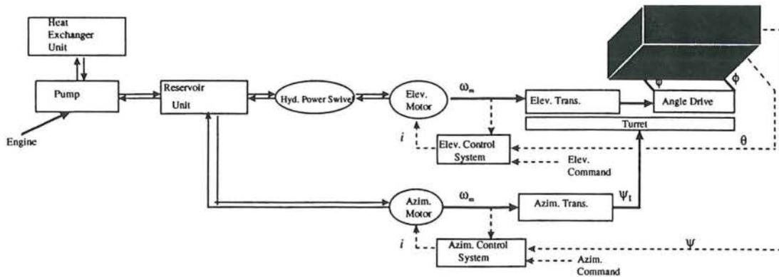
Figure 3: Simplified ILMS Block Diagram
