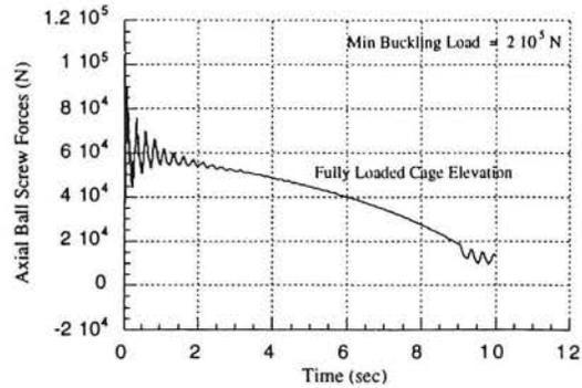
Figure 5: Ball Screw Actuator Forces
