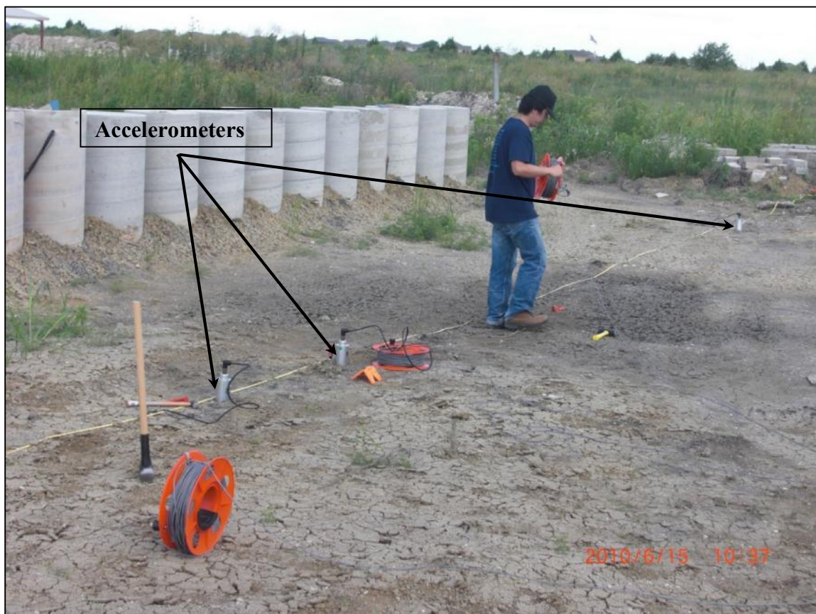
Figure 6.5: Spectral analysis of Surface Waves measurement setup
