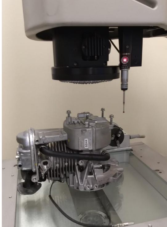
Figure 53: Measuring the mounting hole and crankshaft locations of the GX35 on the Mustang 60 CMM
