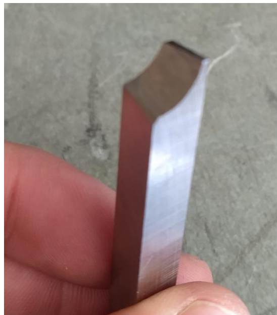
Figure 59: The custom groove cutting tool
