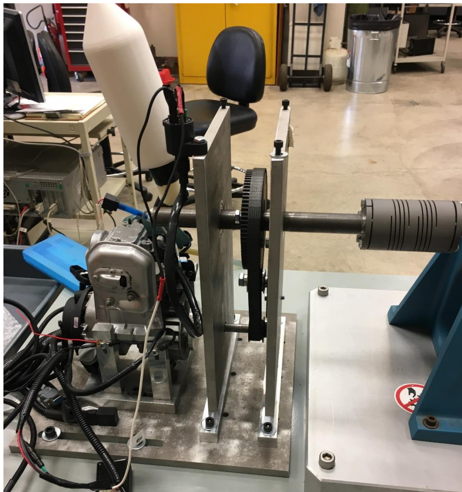
Figure 65: Engine Configuration as coupled to the dynamometer
