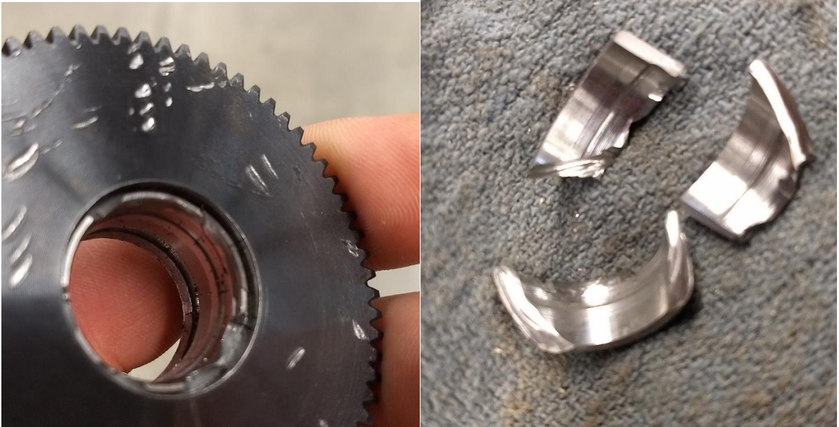
Figure 58: The gear with the remains of the outer race in the bore (left). Marring on the face of the gear was from the vise while attempting to remove the race with a drift. The pieces of the race after slicing and removal (right).
