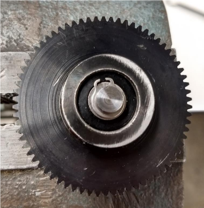
Figure 61: The gear and adaption shaft with the retaining c-clip
