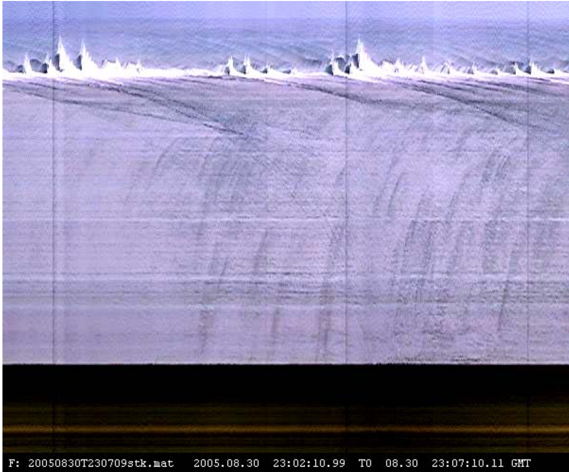
Figure 7. Non-rectified timestack. Date is Aug 30 th , 2005. Timespan is exactly 5 minutes. The horizontal and vertical axis corresponds to time and distance, respectively. A quantitative measurement of distance cannot be directly read from this image, as it has not yet been rectified to spatial coordinates. This figure is shown to illustrate the various features detected using video. Foremost are breaking wave heights. Bores are seen adjacent to the broken wave, eventually reforming into secondary swell as they propagate across the reef, as well as reflection from shore. Offshore swell is also evident.
