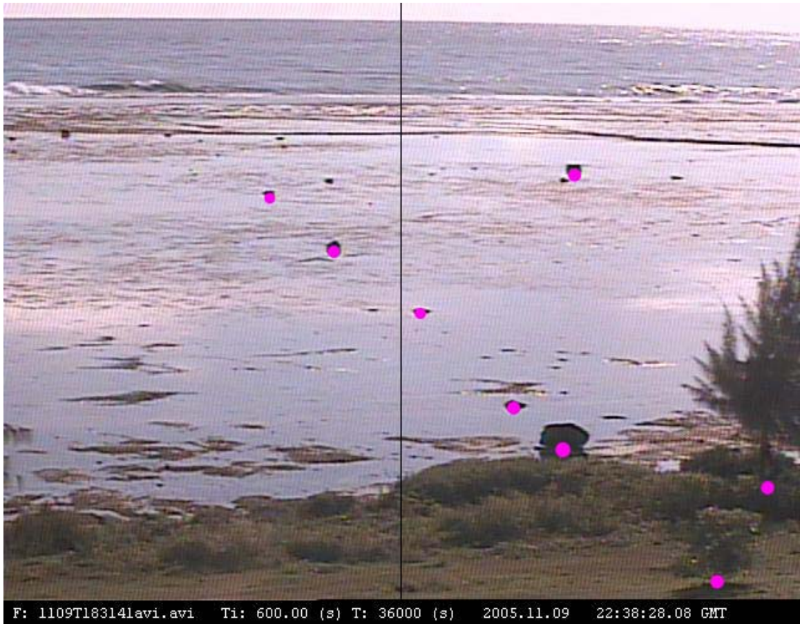
Figure 3. Surveyed ground control points (GCP-s) used in calibration of the camera model. Colored dots are corresponding image coordinates ( u, v ). Vertical black line coincides with image pixels sampled for timestacks.
