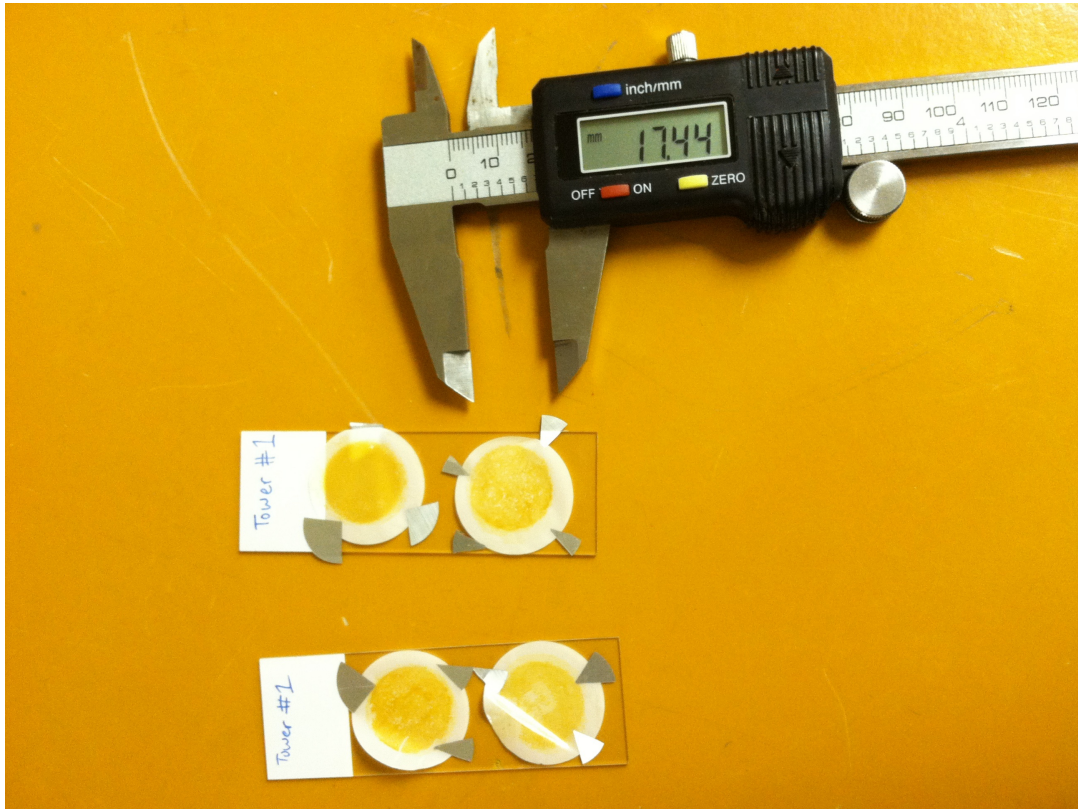
Figure 9: Digital calipers and filters stained with iron oxide solution (photo: Guss)
