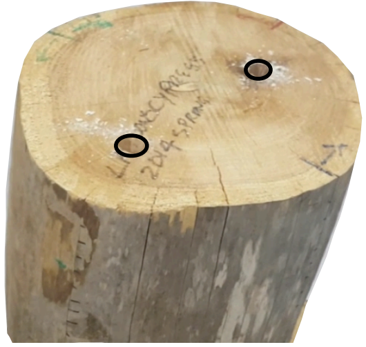
Fig. 4. The tree sample used for the laboratory experiment. The drilled holes are highlighted with black circles.
