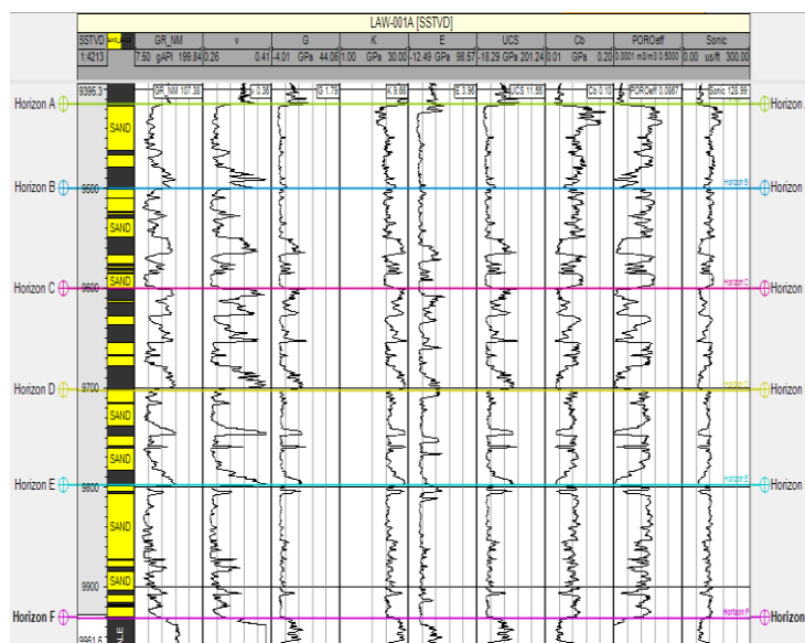
Fig. 5: Geomechanical properties logs showing lithology, poisson ratio ( \nu ), Bulk modulus ( K ), Shear modulus ( G ), Young modulus ( E ), the unconfined compression strength (UCS), Bulk compressibility ( C_b ), effective porosity, compression velocity ( V_p ) of the Law 001A.
