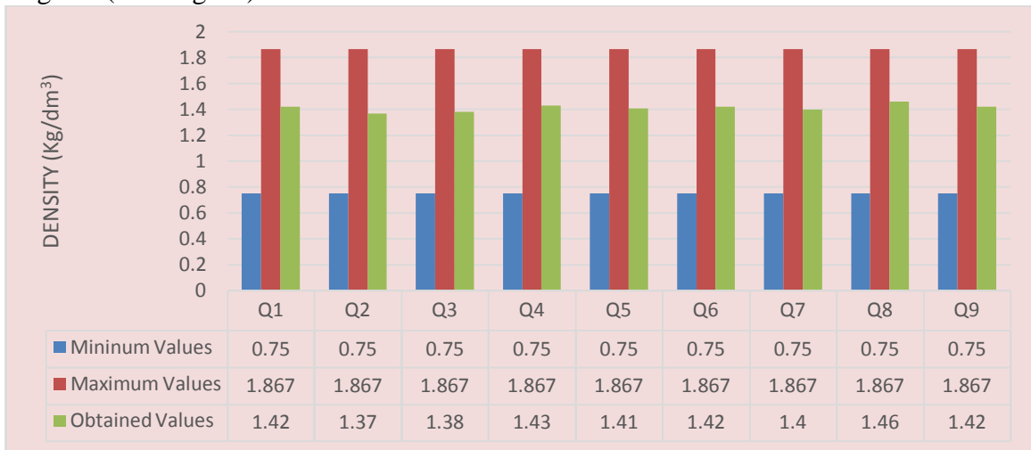
Figure 3.1: Graphical Representation of Sampled Aggregates Loose Density
