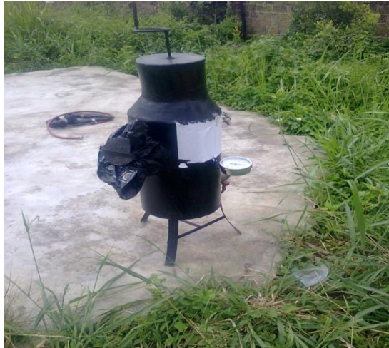
Plate 2: An improvised waste digester
