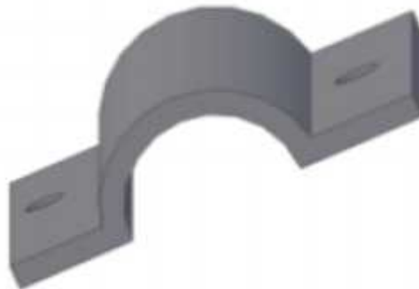
Figure 5: Schematic of fabricated electric motor clip
