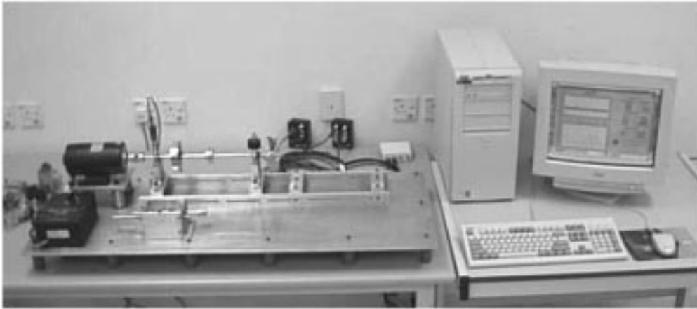
Fig. 2. Setup for automatic fault detection system.
