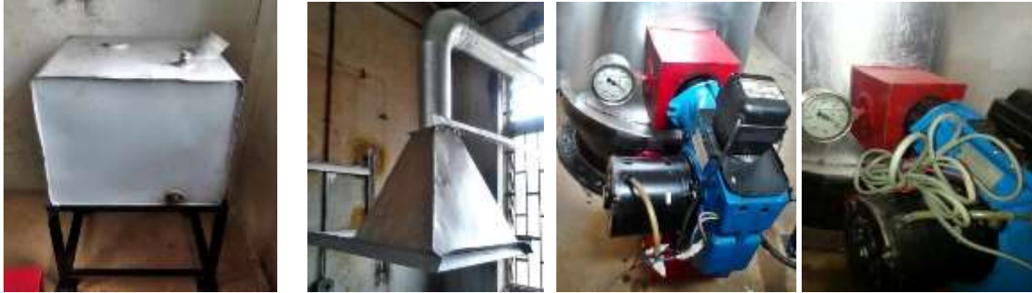
(c) Fabricated Diesel Tank (d) Fabricated Chimney (e) Burner assembly with pyrometer Fig. 3.2: Crucible furnace components.
