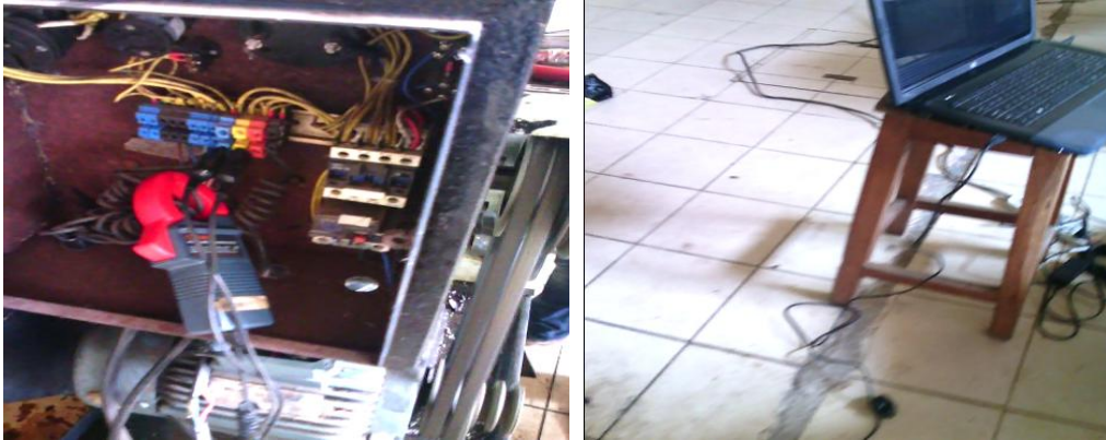
Figure 6: Logger Connected to the Centre Lathe via Electric Motor and Computer System
