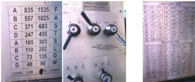
Fig. -3: (a) Selected Cutting Speed (rpm) (b) Selected Feed Rate (mm/min)
