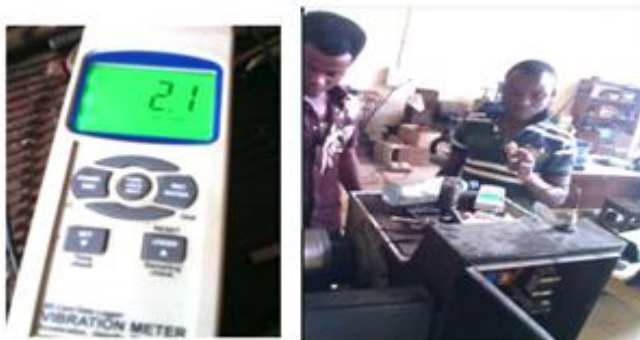
Fig. -5: Portable Digital SD Card Data Logger Vibration Meter (VB 8206SD)
