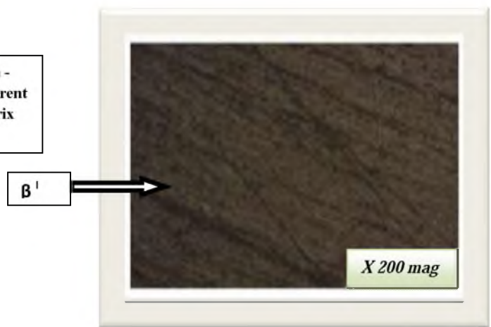
Plate 7: Al 9.37-Cu artificially aged at 500 degree celcius
