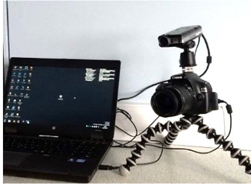
Figure 4.1: Pico Scan structured light 3D surface scanner
