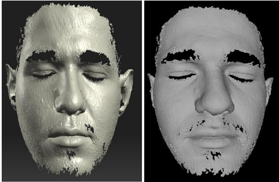
Figure 6.38: 3D geometry of subject with facial hair in HP 3D scan software (left) and MeshLab software (right)
