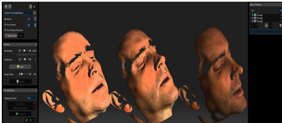
Figure 6.52: Left scan with correct aperture and right scan with the smallest aperture (Alienwaire computer)
