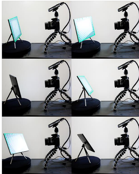
Figure 4.7: Calibration board recorded in different positions
