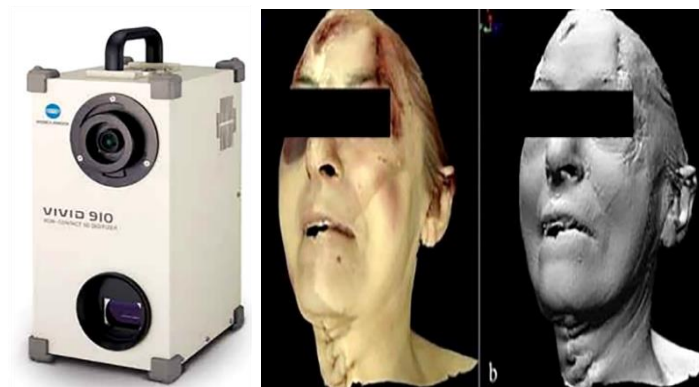
Figure 3.14: Konica Minolta 3D laser scanner and model created by the scanner 26
