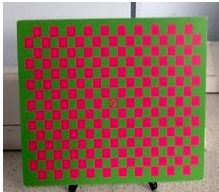
Figure 4.6: Calibration board of the Pico Scan 3D scanner
