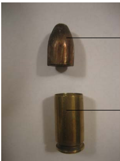
→ Bullet (This is the projectile that is fired from the cartridge) → Cartridge Case (The ammunition casing that is either expelled from the firearm or remains in the chamber after firing)
