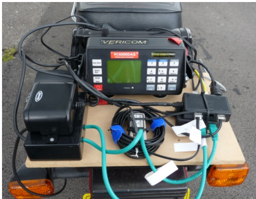
Figure 22 Vericom VC4000DAQ mounted on the rear of the test motorcycle
