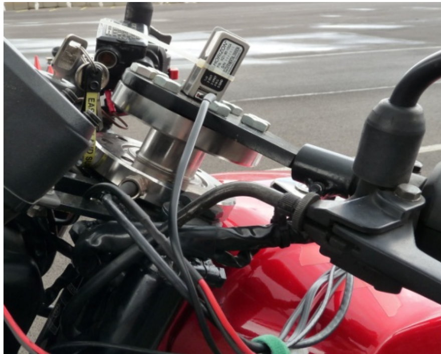
Figure 21 Steering rate sensor mounted above the torque transducer
