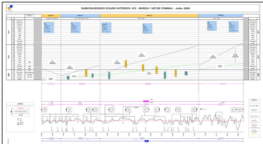
Figure 7.22 Company-produced time-location plan of a 7 km road section (See enlarged image of Figure 7.22 on page 174 for more clear information)
