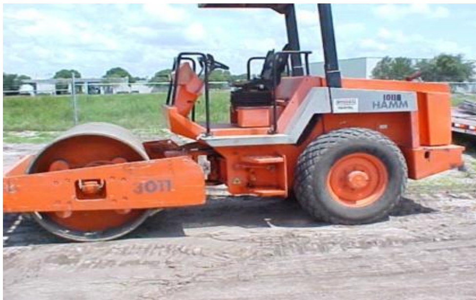
Figure E-2: Compacting roller
