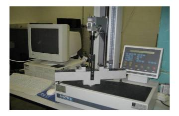
Figure 10. LLOYD Universal test machine
