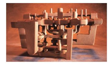
Figure 1. Example of a complex sand core <sup>(9)</sup>
