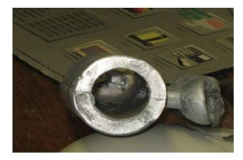
Figure 51. Trial 1B core leached by dilute citric acid (1:1) at 200 °C.
