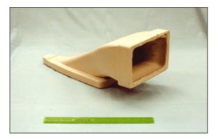
Figure 3. Preformed core for an racing car exhaust component <sup>(10)</sup>
