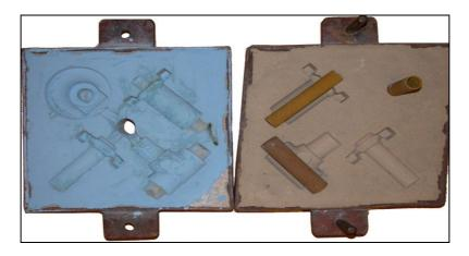
Figure 7. Sand casting with sand cores <sup>(59)</sup>
