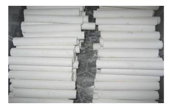
Figure 16. Cores left to dry
