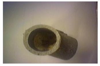
Figure 26. Effect of diluted nitric acid on Trial 1E core fired at 400 °C under
