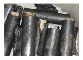
Figure 50. Al-LM25 attacked by dilute potassium hydroxide.
