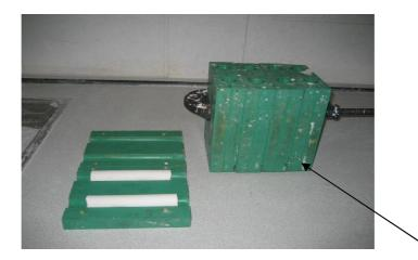
Figure 29. Vertical standing wooden core boxes with cores
