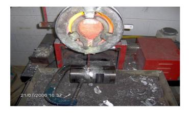
Figure 13. Pouring process to assembled mould
