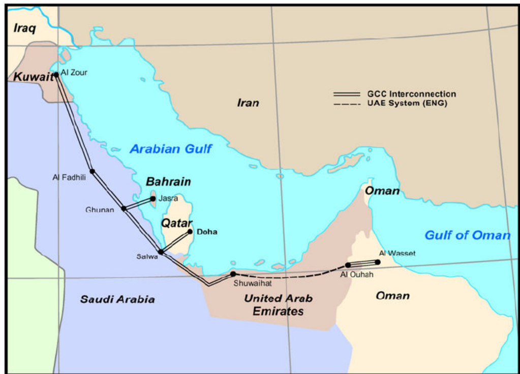
Figure 14.2: Approximate route and layout of GCC interconnection
