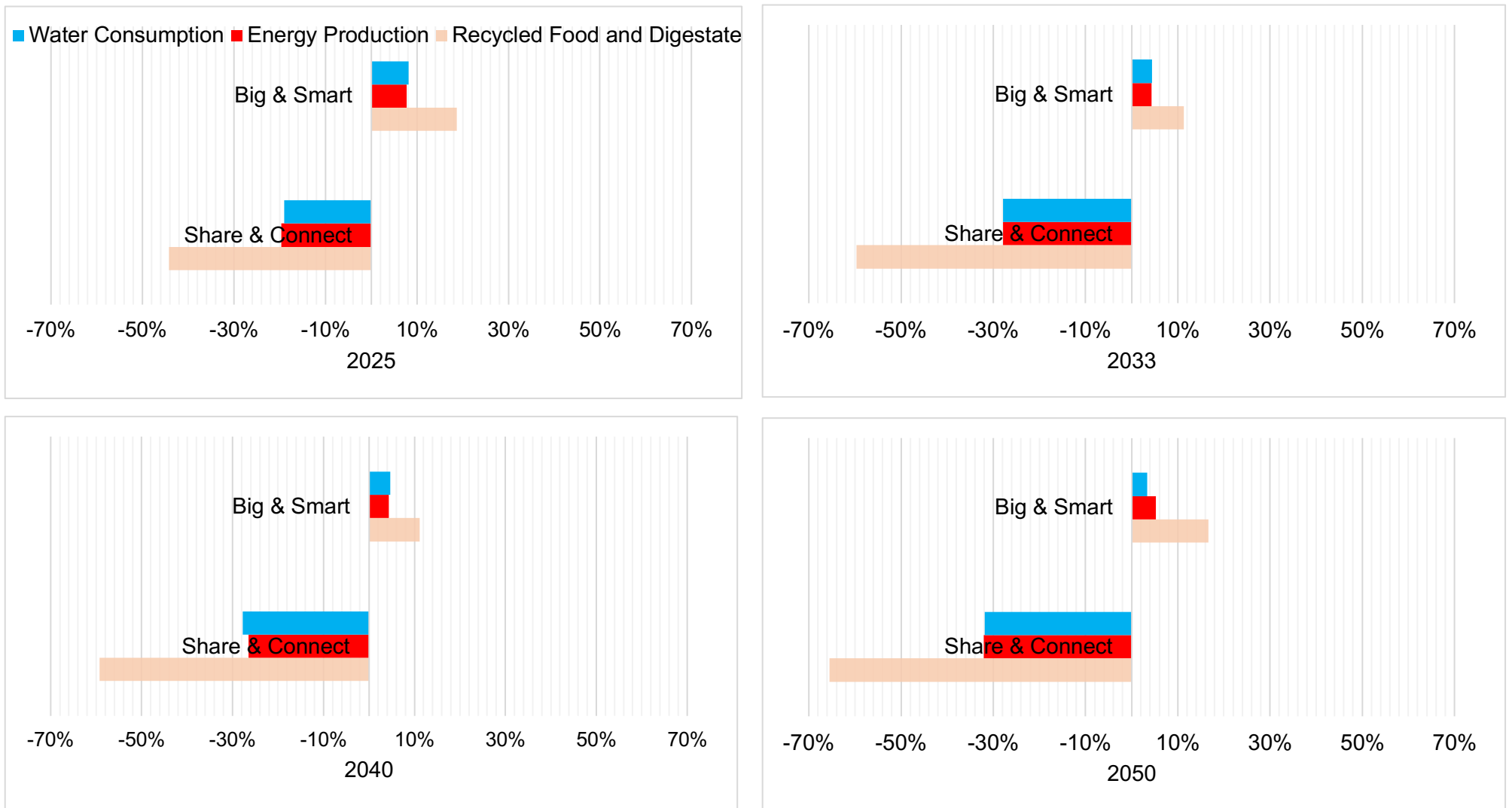
Figure 13: Variation of impacts on the Water Energy Food nexus in years 2025, 2033, 2040 & 2050 compared to Baseline (Equations 5, 6 & 7). Negative percentages indicate lower values than Baseline.
