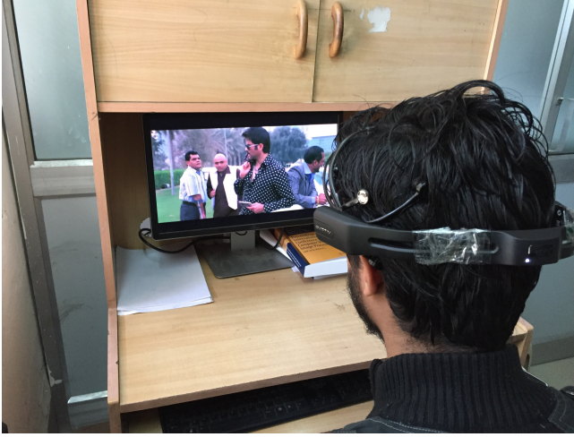
Fig. 5 A subject watching a video while wearing EPOC Emotive Device (EEG Device setup).
