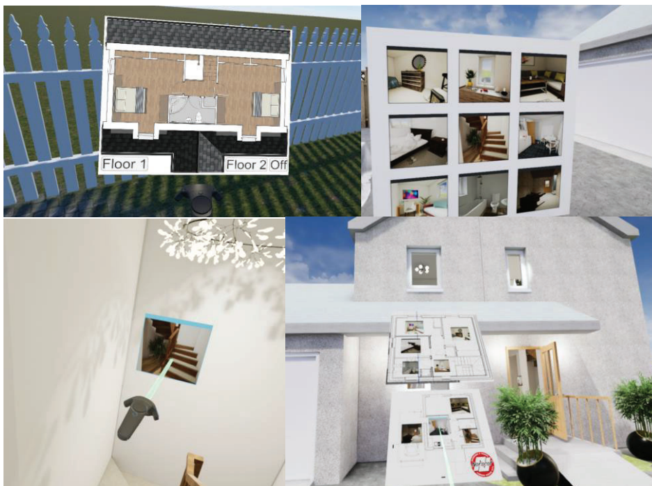
Figure 3: Floor Plan Visualisation. Left to Right: Floor Plan Attached to Left Controller; Reusable Teleport Buttons System; Aligned Floor plan.
