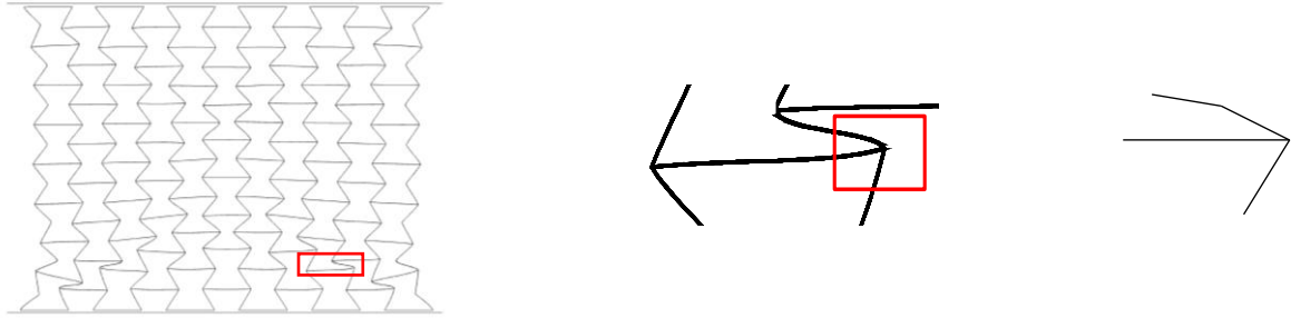
Fig. 8. A typical localized deformation patterns of these honeycombs with the strain of 0.1
