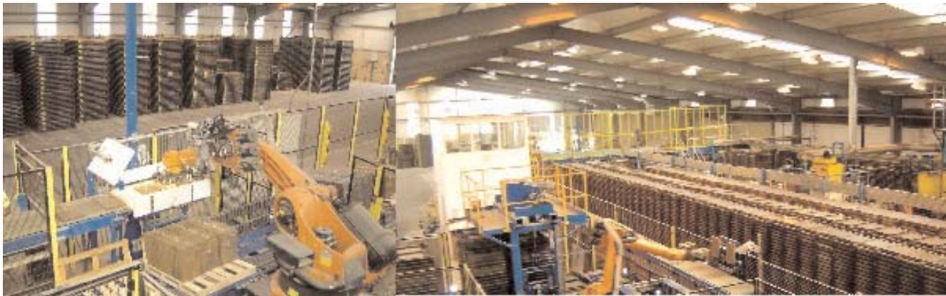
Figure 5: Pallet Building Robot – Vision enabled
