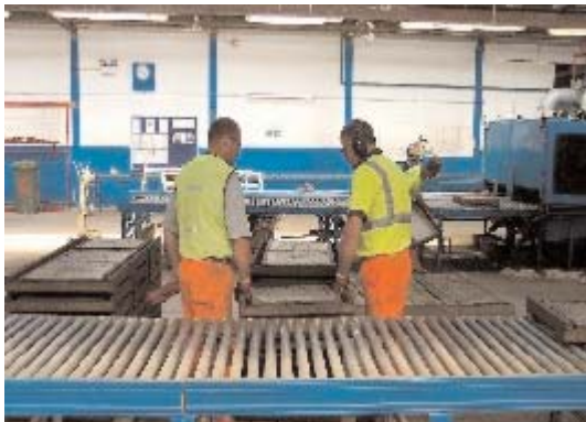
Lifting Off – Filled Mould
