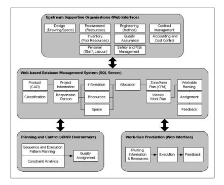
Figure-2: LEWIS System Architecture
