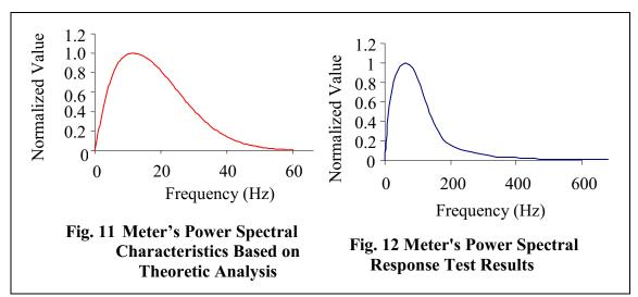
spectrum bandwidth is narrower. However, the similarity between the two figures is apparent, generally confirming the above assumptions.
