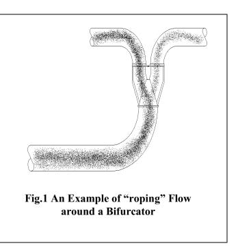
their studies, it was concluded that the solids can undergo inhomogeneous concentration distributions across a given pipe cross-sectional area. Such distributions are affected by the conveyance velocity, particle size, humidity, and conveyor geometry. The so-called "roping" flow regime is an extreme example of inhomogeneous distribution where inside the "rope", the highly concentrated solids flow is formed, as illustrated in Fig. 1.
