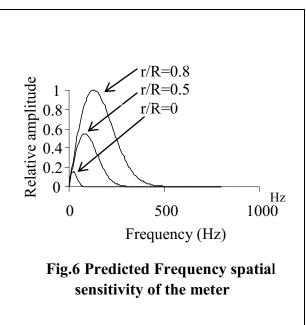
the fluctuation in the net charge. The "flow noise" is usually regarded as a band-limited white noise, as is the fluctuation in net charge  $q_{NETr}^{P}(\varpi)$ . Figure 6 shows the predicted
