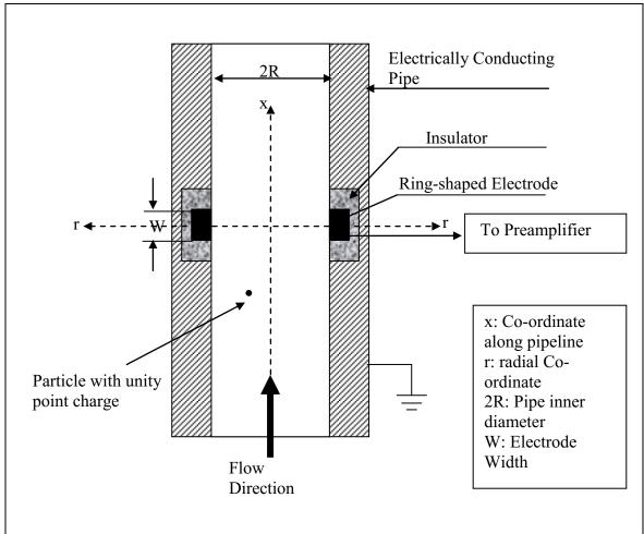
earthed conveyor. The electrode is insulated from the conducting conveyor wall but exposed to the flowing air-solid mixture and is ac coupled to an amplifier.
