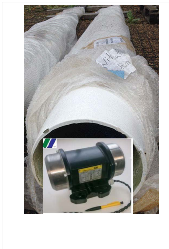
Fig. 11: Turbine blade mock-up and mechanical shaker
