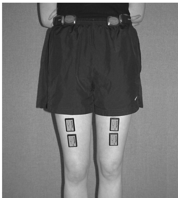
Figure 2 The monitors in position for testing. The activPAL monitor is worn on anterior mid-thigh, and the pedometers placed on the hip with the Omron lateral to the Yamax. Informed consent was obtained for publication of this figure.
