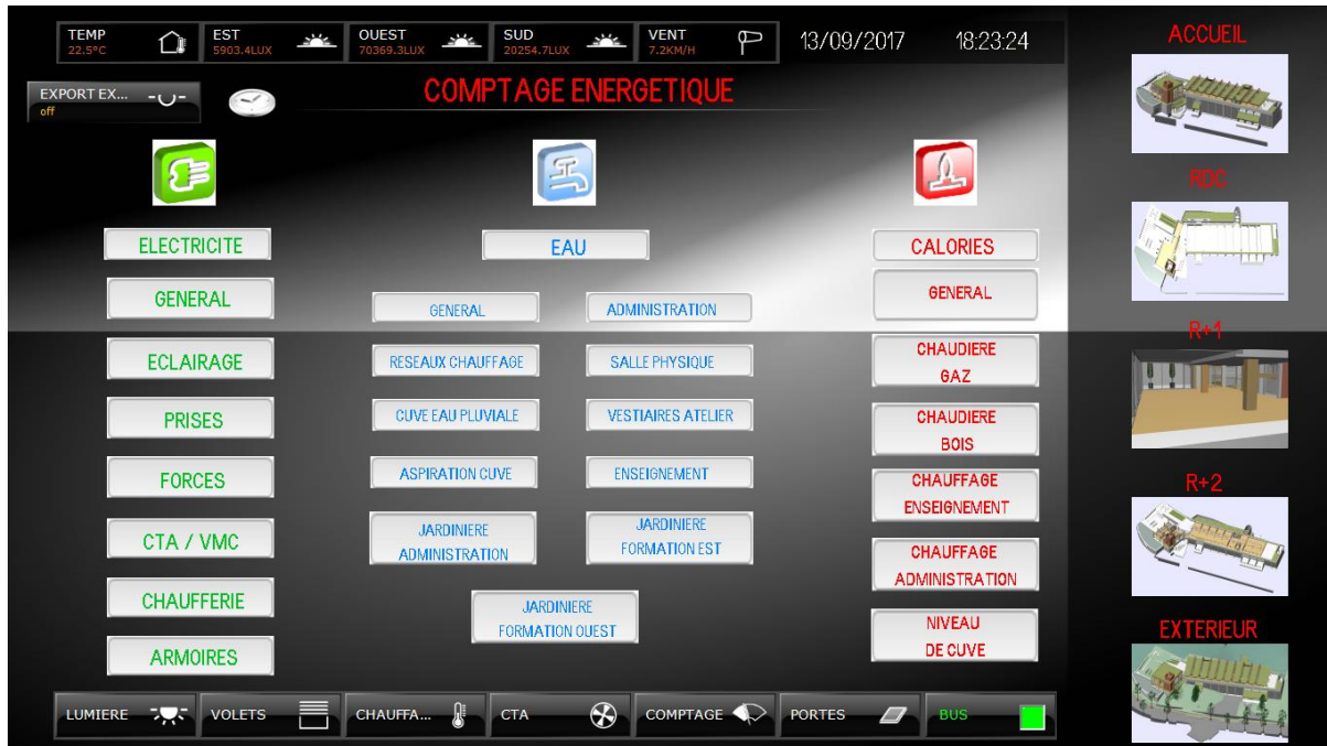
FIGURE 30. ENERGY METERS SCREEN INTO THE FCMB BMS
